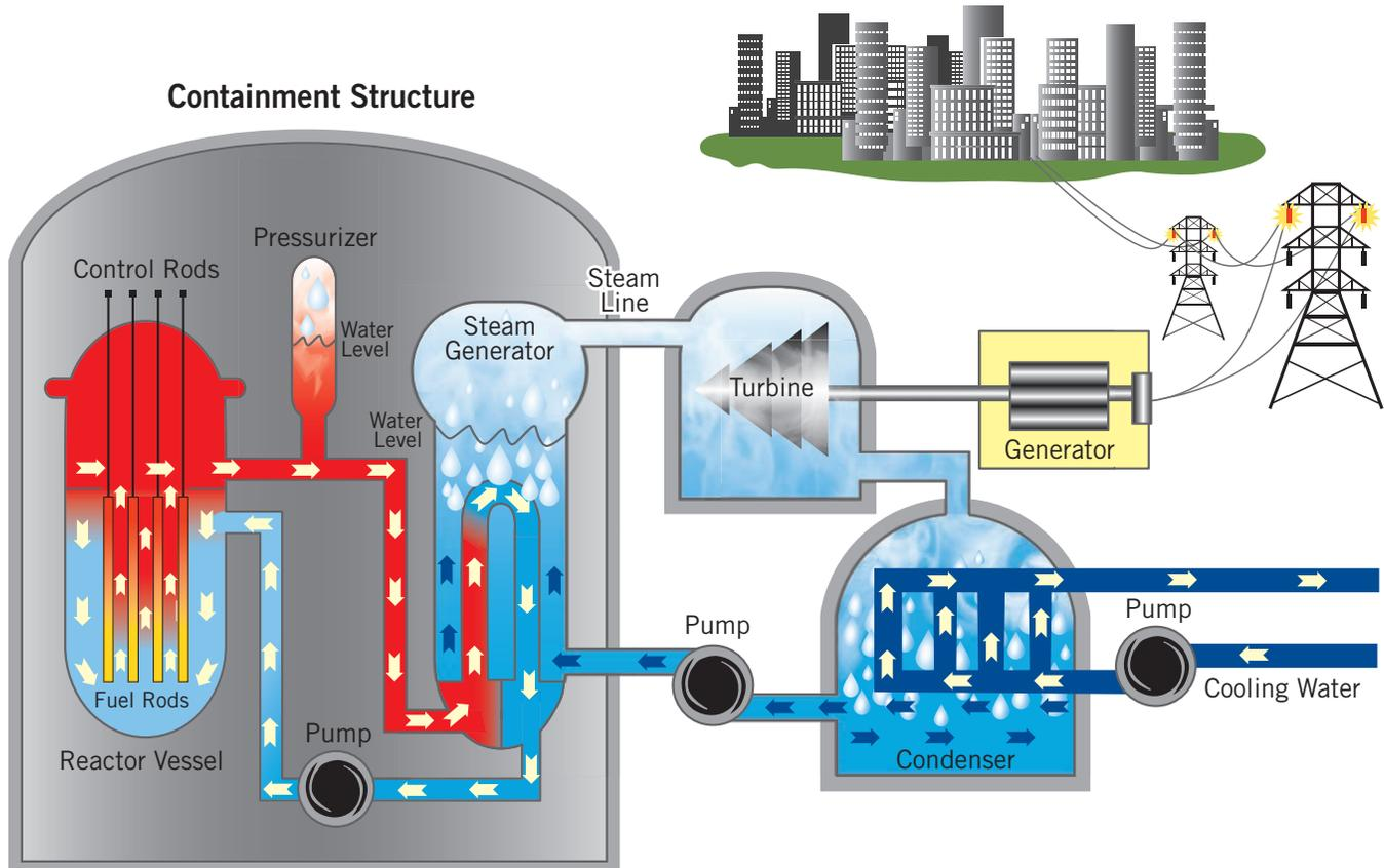
The steam exits the turbine and then passes through a condenser, where it is cooled by cold water from a cooling tower or another source, such as a lake. When cooled, the steam condenses to liquid water and is returned to the reactor core to begin the process again.
